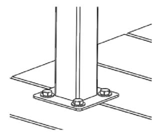
Fortress Posts must always be secured to the deck framing and should never be attached to only the deck boards.
